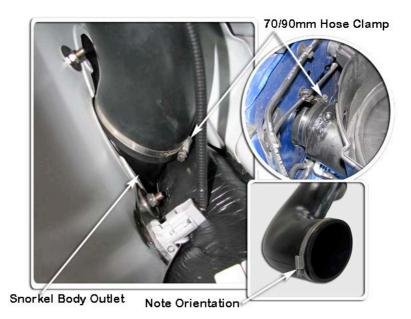
Install the black hose clamp (Item 14) loosely over the base of the air ram assembly (Item 2).
