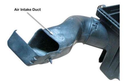
Remove and discard the air intake duct.
