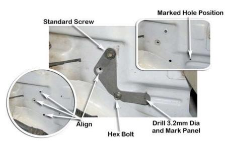
Use a centre punch to punch the centre of the hole accurately, this will ensure the drill stays central whilst drilling.
