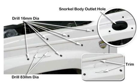
Hex Bolts Install the upper mounting **Upper Mounting Bracket** snorkel body (item 1) with Apply loctite 243 to each of the stainless steel mounting studs (item 6) and install the studs finger tight into the
