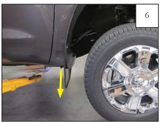
Remove push retainer from underside of factory mud guard. Remove Mud Guard from Vehicle.
