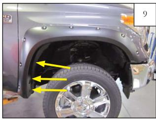
Start three supplied 20mm Hex Screws (SW1-0036) through three rear holes in flare and into factory holes in rear of wheel well.
