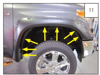
Ensure flare is properly positioned and tighten all screws. (Repeat for other side of vehicle) Installation Comlete.
