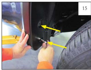
Start two supplied 20mm Hex Screws through the rearward most holes of flare and into the factory hole in fender.
