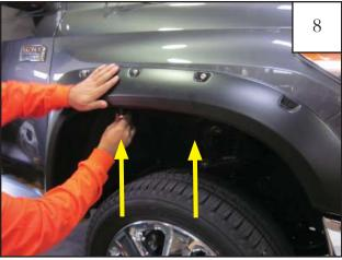
Place flare on fender, alighning holes with clips on the bracket. Start two supplied 20mm Hex Screws (SW1-0036) throught two holes on the top of the flare and into clips.
