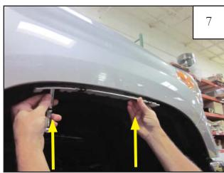
Using two supplied 20mm Hex Screws (SW1-0036), attach bracket to factory holes with a 10mm socket.
