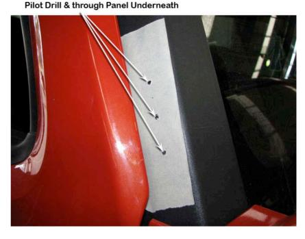
Remove the A-pillar plastic trim and apply a strip of protective cloth tape or similar along the door leading edge to prevent damage to the door frame.
