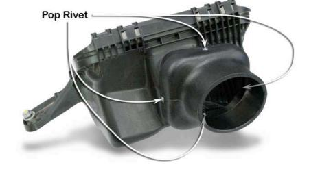
Re-install the air cleaner base as you guide the adaptor duct entry (Item 3) into the air entry hose (Item11).
