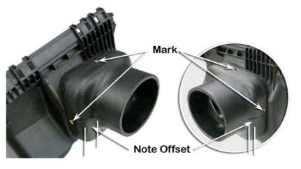
Apply Sikaflex sealant to the outer surface of the air cleaner base inlet.
