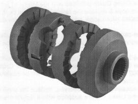
The springs simply sit in their final positions in the cam gears. The pins (already fitted into the cam gears) with the stepped end exposed, are positioned as the one cam gear is placed onto the second cam gear. The stepped end simply sits into the end coil of the spring and pushes harder onto the spring as the 2 carrier 'half' assemblies are bolted together.
